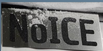
Black icephobic thermally sprayed coating on steel substrate under icing conditions.
