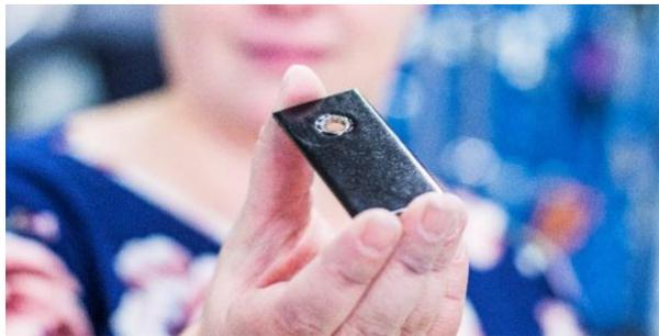
Picture 2. Example of thermally sprayed icephobic polymer coating. Photo: Jonne Renvall/TAU.
