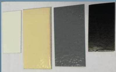
Color of icephobic thermally sprayed coatings can be tailored by feedstock materials.
