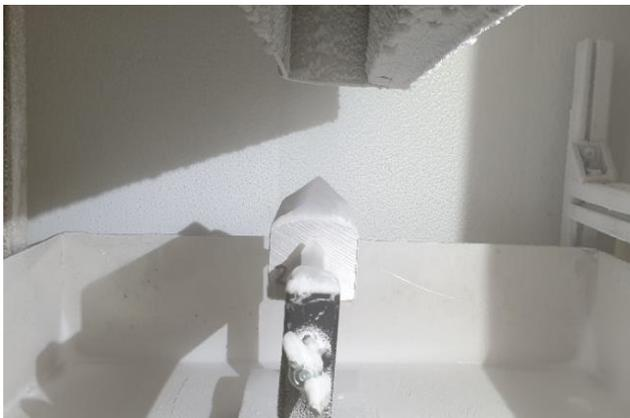
Figure 2. Train profile sample under the icing wind tunnel.
