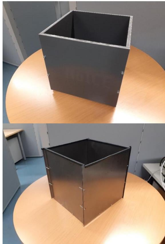
Picture 1. Test boxes, 1) PE 2) Steel
