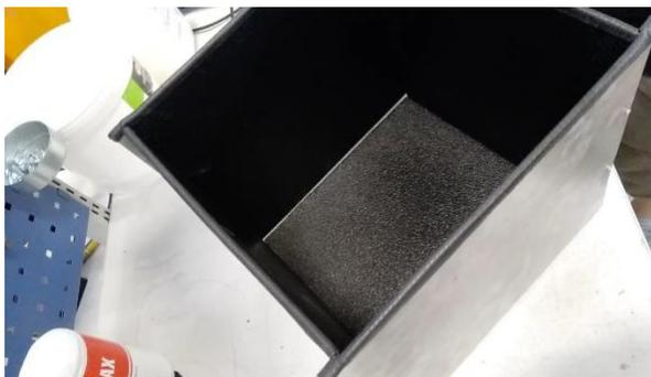
Picture 3. Coated box with FS-PE
