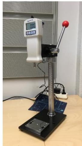
Picture 4. Shear test installation
