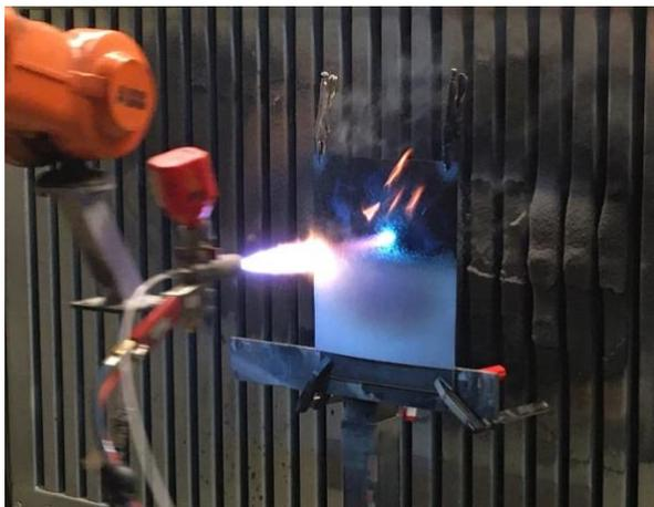
Picture 2. Coating in progress at Tampere coating lab
